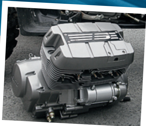
Drysdale's inline three-cylinder engine that powers the Vento ATV
