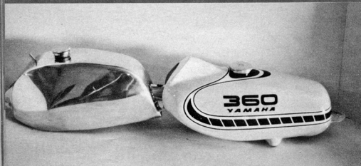
Two of the best tanks on the market are Torsten Hallman's aluminum works tank at 3½ lb. and the Jones Motocross Products fiberglass replica of the YZ tank at 2½ lb. Both offer excellent quality.
