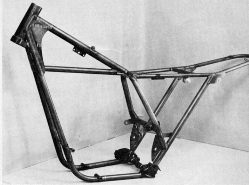
The Champion motocross frame is constructed entirely of chrome moly tubing. Extremely strong, with a proven geometry for excellent handling, it weighs only 17 pounds.
