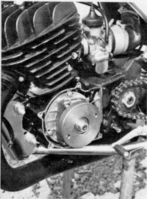
Torque wheels are one of the most important items to smooth out the powerband of the Suzuki. The units are available in 1¾, and 2¼-pound sizes.
