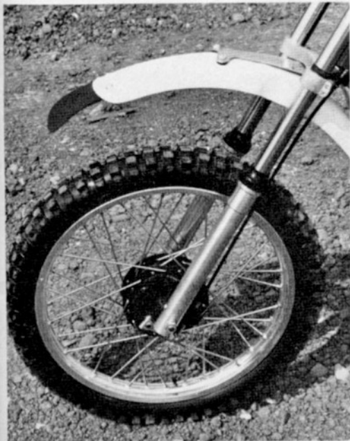
If good forks allow a rider to ride 5 mph faster than regular forks, then Cheney forks allow him to ride 10 mph faster. The $300 price puts them out of reach of most of us, but they are probably the finest forks you can buy. Front hub is standard Suzuki, rim is DID, front tire a Trelleborg.
