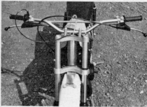
Cheney fork crowns are made of cast aluminum and weigh only 4¼ pounds, including the fork stem. Handlebars are made of heat-treated chromoly and weigh only 1½ pounds. Throttle is "El Cheapo," from a Yamaha DT2.
