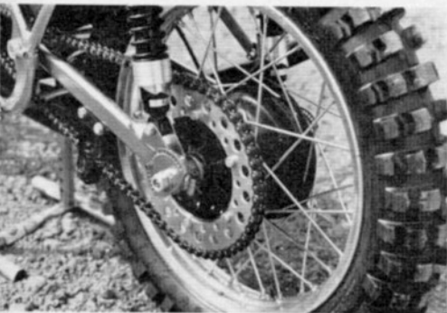
The rear wheel assembly weighs about 28 pounds. Cheney axle adjusters are foolproof. Upper shock mounts allow slight side play and let you remove springs by simply unscrewing top retaining screw.
