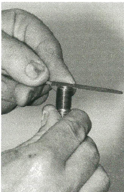
No detail is too small. Todd manicures the threads at the end of each rod.
