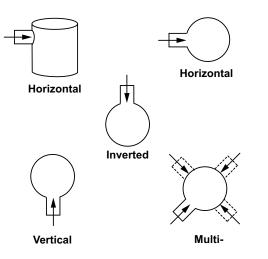
The qualified positions listed include only those tested. In some cases, the manufacturer may claim other positions, but test information at this time neither support or refute such claims. An arrester tilted more than 60 degrees from its qualified operating position may not adequately arrest sparks. Therefore, arresters on mobile equipment—other than screen type arresters— shall not be mounted more than 45 degrees from the qualified position. See column marked "Appl Pos."
