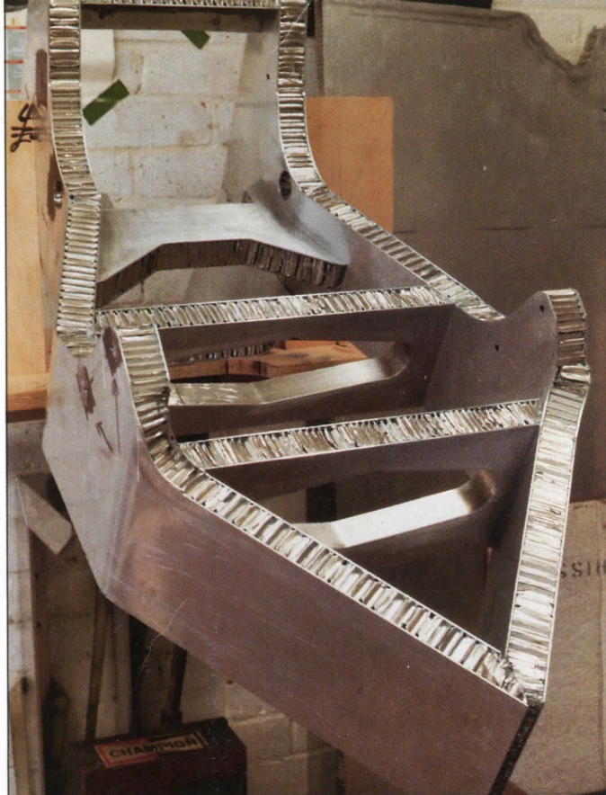
Shaped honeycomb board reveals thin cross-members until pieces of skin are glued into place along open sides
