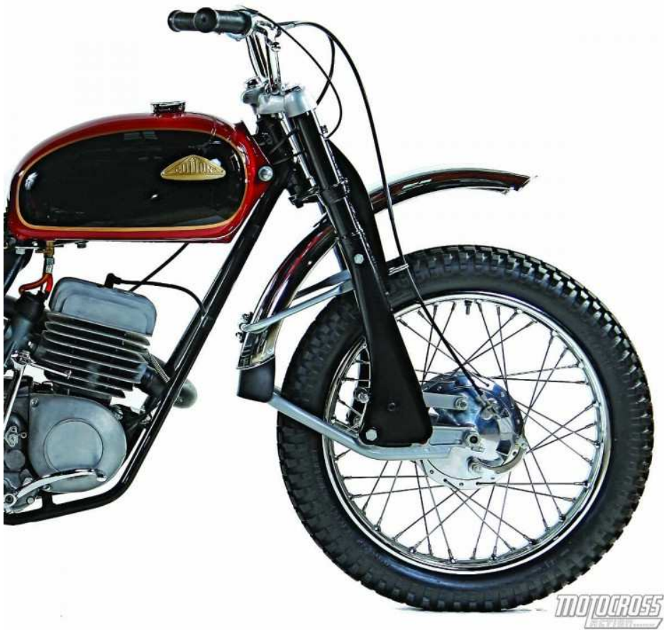
The Cotton Cobra came equipped with Armstrong leading links.
