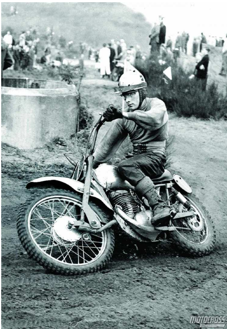
The late Dave Bickers on a leading link Greeves (with an aluminum frame).
