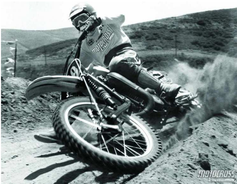
MXA test rider Lance Moorewood rails a Saddleback berm in a 1980 Yamaha YZ250 outfitted with Thorks and a Fox air shock. The shocks on the forks are by S&W.
