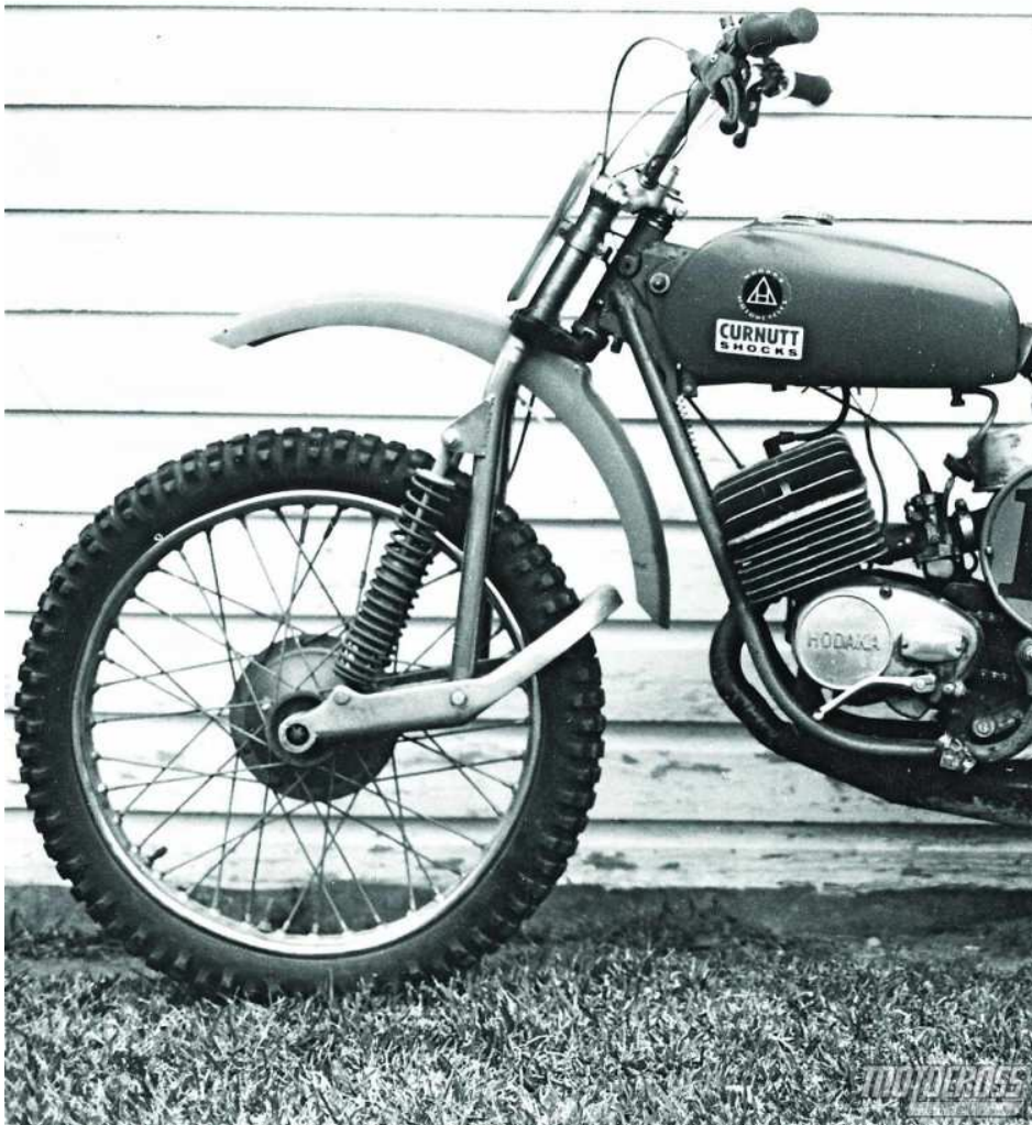
Jody's Hodaka Super Rat ran Swenco leading link forks. The Swenco forks were an aftermarket bolt-on that used the stock triple clamps to hold the chromoly fork legs. The front swingarm was cast aluminum. Jody preferred Curnutt shocks (front and rear).
