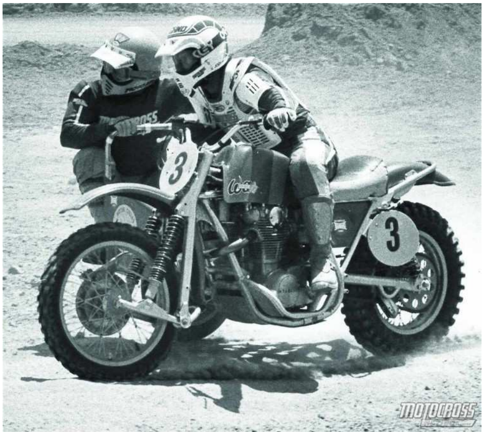
Most sidecarcross bikes still use leading links to hold up the mass of a big bore engine and two men. Here, Jody Weisel powers a Yamaha 650 twin engine Wasp to second in the 1983 California Sidecar Championships.
