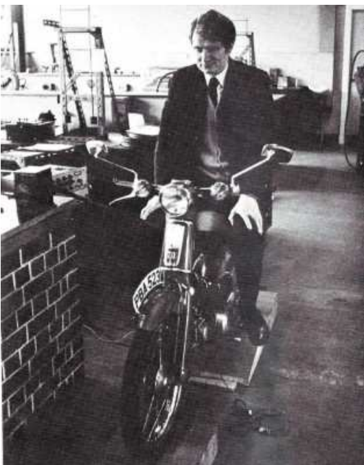
Dr Terry Thorpe on the Honda 90 step-through which was handed to them for evaluation by the (British) Road Research Laboratories. The discovered it was unstable above 45 km/h, but because of the low mass involved it was relatively unimportant.
