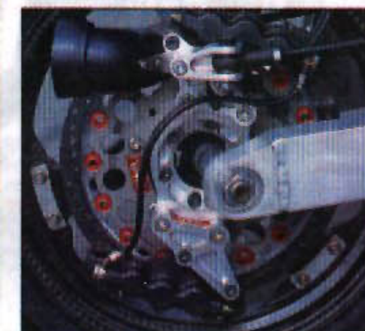
HUGE BEAST: 310mm brake disc and calipers
