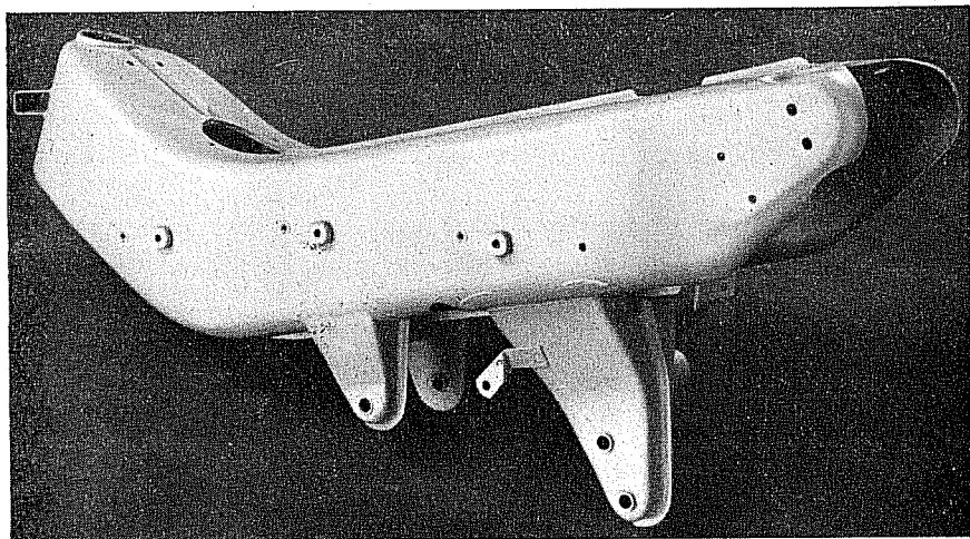
Fig. 3 (right).—Main frame complete with engine-mounting brackets
