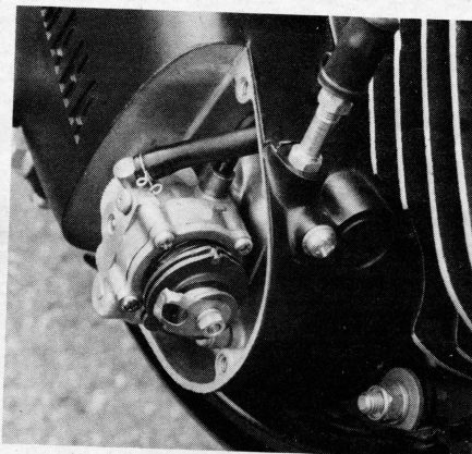
Cover removed to show oil pump on production bike. Convenience overshadows weight factor.
