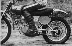
Under acceleration note deflection of the rear tire (pumped to 12 lbs. p.s.i.) as indication of just how much drive is being obtained.
