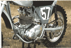
Weight concentration is down low. Pursing chassis just clears BSA oil drain plugs for easy service
