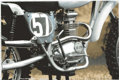
Pursang chassis was stretched to accommodate longer and taller BSA four stroke by relocating swingarm pivot point 20mm to the rear and adding chassis rally tube rear engine mounts
